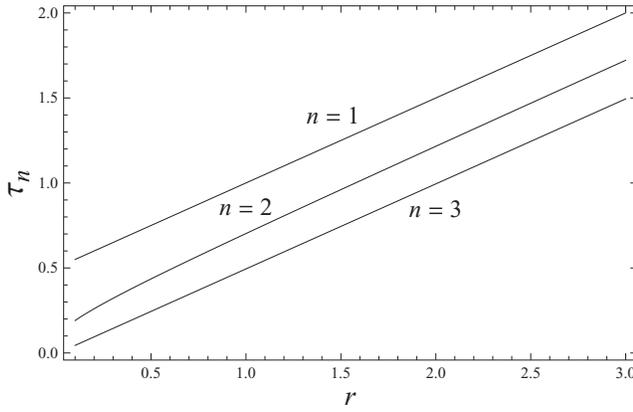
FIG. 1. Dependence of the local accumulation time on  $r$  in different space dimensions obtained from (5), (13), and (17) with  $D = 1$ ,  $k = 1$ , and  $R = 0.1$ .
