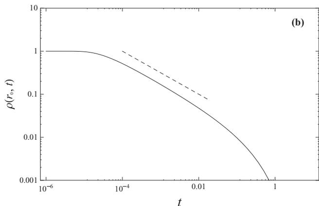
FIG. 5. Dependence of the relaxation function  $\rho(r_0, t)$  on time for  $r_0 = 0.01$  in three space dimensions, obtained from the numerical solution of (3) with  $D = 1$  and  $k = 1$ . In (a),  $\rho(r_0, t)$  is plotted on the linear scale. In (b),  $\rho(r_0, t)$  is plotted on the log-log scale. The dashed line in (b) indicates the  $t^{-1/2}$  dependence.
